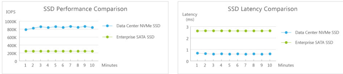
Figure 2: Data Centre NVMe SSDs display significant performance and latency improvement over SATA SSDs
