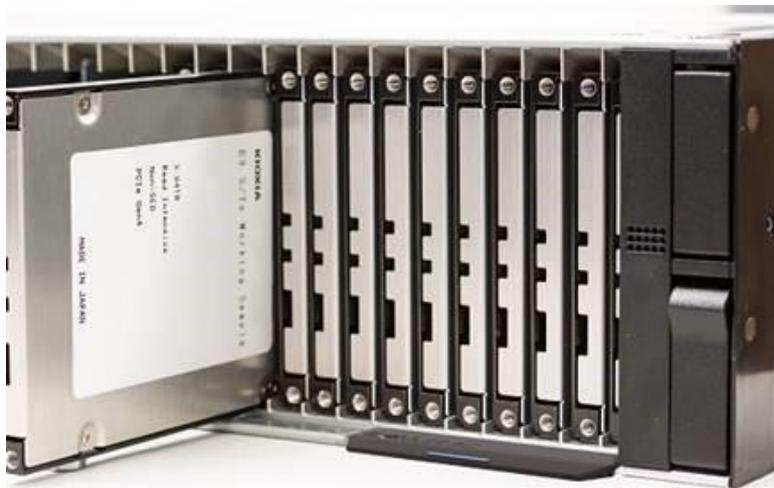
**Caption:** The image shows SSDs mounted on a 2U-size rack mounted server prototype that installs max. 48 units of major server vendor's prototype. With the combination of E3.S evaluation model + 2U rack mounted server evaluation model, KIOXIA has been performing target device evaluations such as system performance evaluation, heat dissipation verification, etc. with server vendors.
